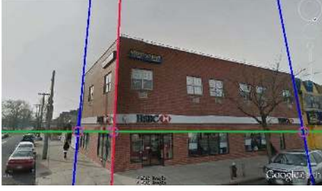
Figure 4: An example of identified vertical corner edges, blue indicated boundary corner edges, red indicates an intersecting corner edge, and green stands for the horizon.
