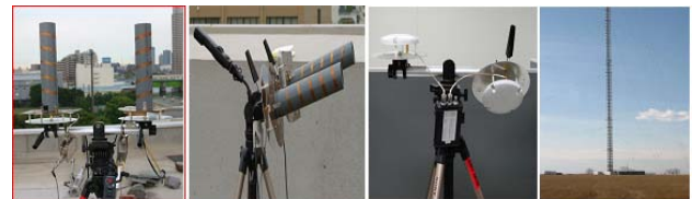
Fig. 2 Different antenna orientation for ground-based observation. (a) Both RHCP and LHCP oriented vertically up (b) Both RHCP and LHCP oriented towards the building surface (c) RHCP antenna oriented towards zenith (sky) for direct signal and LHCP oriented towards ground for reflected signal (d) 300m tall Boulder Atmospheric Observatory (BAO) Tower at Colorado. Data logged in this tower are used for analysis in this paper
