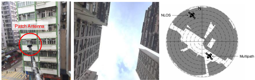
Figure 6. The left panel indicates the installation of the patch antenna, the middle panel illustrates the data collection environment and the right panel indicates the skyplot with building sites used to label NLOS and multipath measurements
