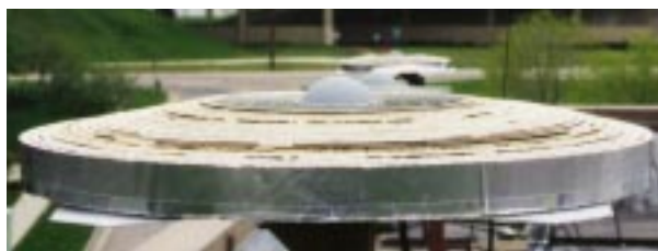
Figure 1. Ground reflected multipath was minimized using choke ring antennas augmented with ring shaped collars 25 cm in width.
