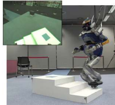
Fig. 1. The HRP-2 humanoid autonomously climbing a set of stairs. Environment mapping and robot localization is accomplished online using our GPU-accelerated 3D tracker (tracker view inset).
