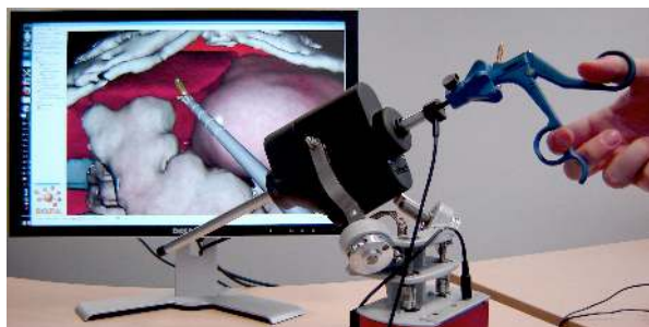
Figure 6: Simulated grasping of the liver using a laparoscopic haptic device. During this interaction, the liver can be in contact with the ribs, colon or stomach.
