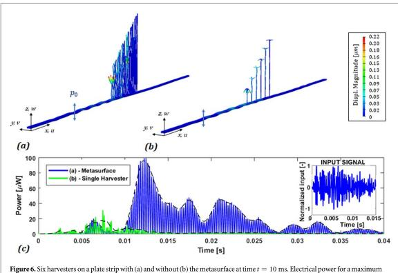
input acceleration of 1g with and without the metasurface (c).
