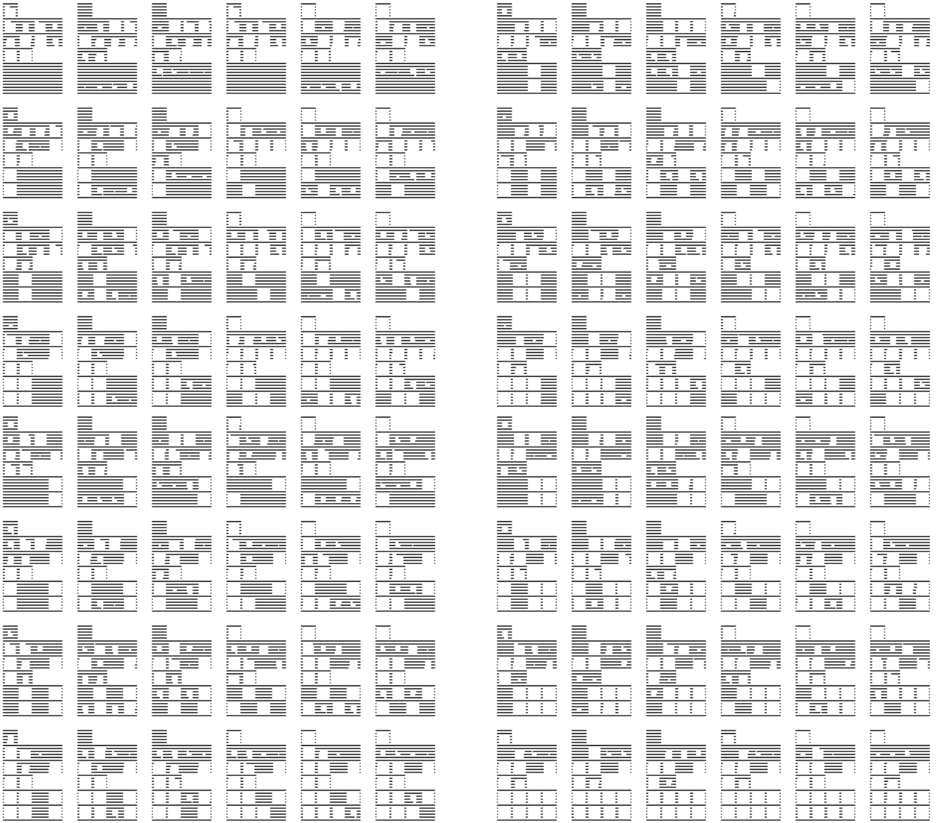
Fig. 4. Network state for all the cases in the four bit rotation problem. This display shows the states of the units, arranged as in figure 2. Each row of six shows one value for register A. There are 2^4 = 16 such rows. Within each row, the three diagrams on the left show the network's state when competing the direction bit, register B, and register A, unshifted. The right three are the same, except with a shift. Note that all completions are correct except in the two cases where the rotation bit can not be determined from the two shift registers, namely a pattern of 0000 or 1111.
