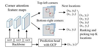
Figure 5: Illustration of corner attention module. Each scale's corner attention maps consist of the top-left attention map and the bottom-right attention map. In the inference process, the center (x, y) of the next location needs to be caculated according to the scale and top-left point or bottom-right point, respectively. Then non-maximum suppresion (NMS) operations are performed together to remove redundancy.
