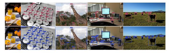
Figure 6: The first row in this figure is the detection result of CornerNet-Saccade with corner pooling while the second row is that with GCP module. The performance of keypoint-based detector is significantly improved with GCP for arrayed objects.
