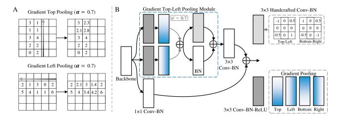
Figure 3: A shows calculated value of the gradient top-left pooling. B shows the pipeline of gradient top-left pooling module. We replace the original corner pooling with gradient corner pooling and add a group of handcrafted convolution kernels after the corner pooling to identify fixed corner patterns.
