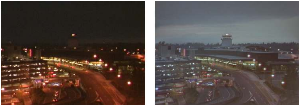
Fig. 1. Enhancing a night-time scene from an airport surveillance camera. A low quality night-time image, and the final output of our algorithm.
