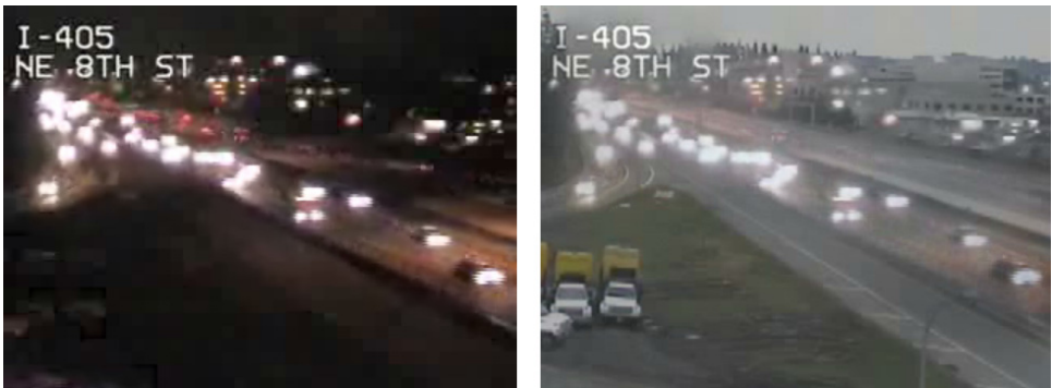
Fig. 2. Enhancing a traffic video. A low quality night-time video frame, and the final output of our algorithm.
