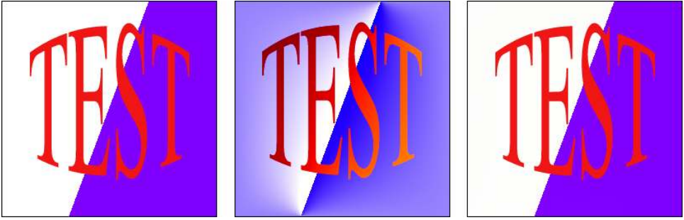
Fig. 4. Overcoming integration artifacts by padding. (Left to right) The original image, the integration result without padding, and the integration result using padding.
