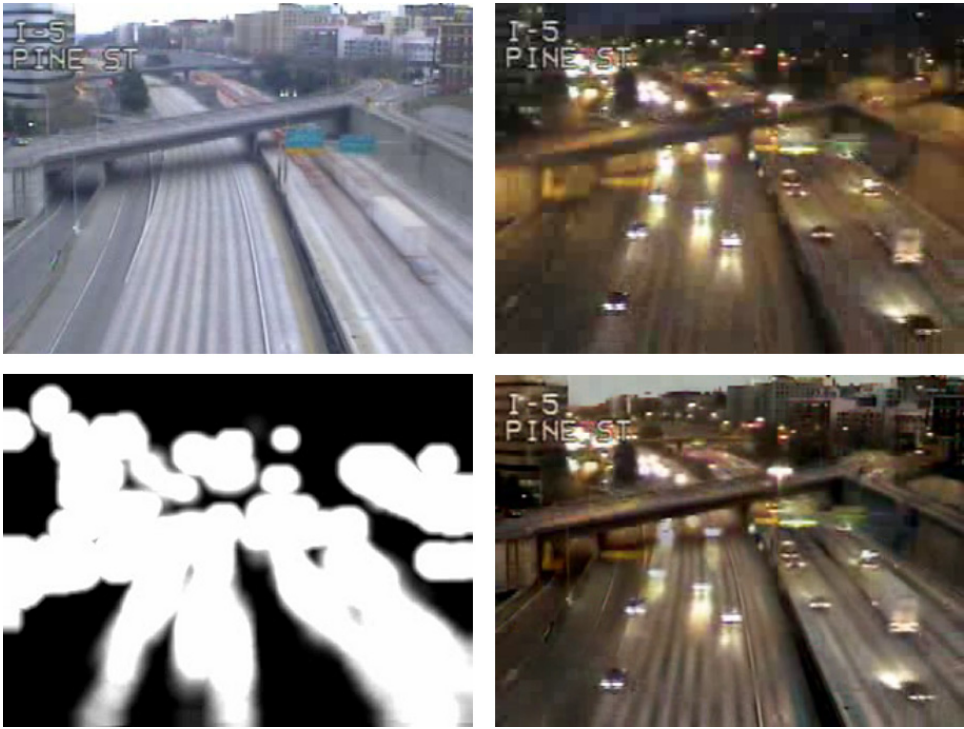
Fig. 8. Enhancing traffic video. (Top row) A high quality daytime and a low quality night-time video frame. (Bottom row) The importance image obtained after processing, and the final output of our algorithm. Notice the road features and background buildings.
