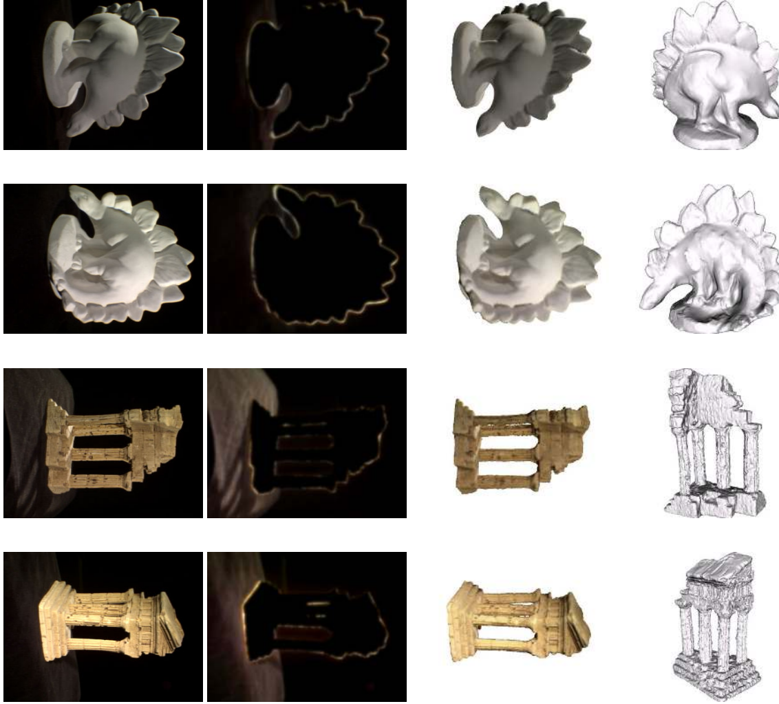
Fig. 9 Dino and Temple sequence (input data courtesy of [36]). From left to right: 1 of 16 input images; estimated background images (scaled by 2 for visualization); estimated radiance; estimated mesh seen from a different viewpoint.
