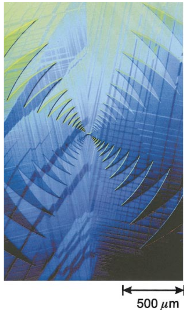
FIG. 75. Phase contrast micrograph of a Josephson junction with a logarithmic-periodic antenna on a \text{LaAlO}_3 bicrystal substrate. The vertical grain boundary in the middle of the picture and the twin boundaries in the substrate can be clearly seen. The size of the image is 2370 \times 1550 \mu\text{m}^2 . From Kaestner et al. (2000); figure courtesy of M. Schilling, Universität Hamburg, Germany [Color].
