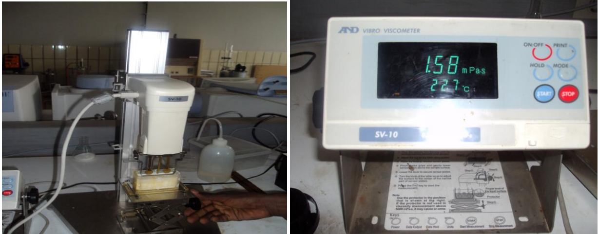
Figure 3. Vibro Viscometer (Model SV-10, Switzerland, 2007)
