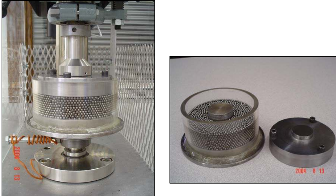
Figure 9.2 : Shear Cell Assembly
