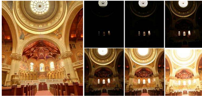
Figure 2: Example of generating HDR image from multiple exposures. Image courtesy of J. Levenson
