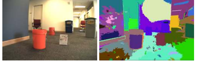
(a) The camera image for the ‘hallway’ dataset. (b) 2D segments extracted via image-only segmentation from [3].
