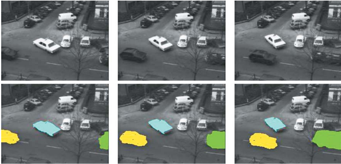
Figure 9. Segmentation of a video sequence (21 frames). Initial segmentation takes 3–5 seconds while correcting seeds are incorporated within a second. The car in the center is the simplest to segment. It is enough to place hard constraints (seeds) in one frame. The car on the left required some editing due to low contrast and seeds were placed in 3 frames. The bus on the right moves behind a tree and its segmentation required seeds in 4–5 frames.
