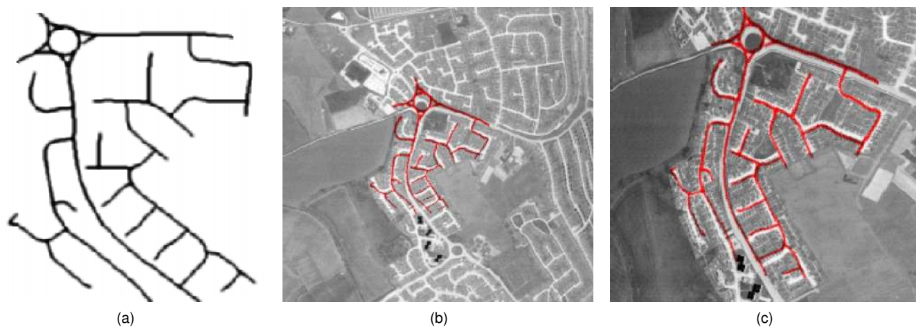
Fig. 13. Aerial image registration. (a) The digital map. (b) The registration with the high altitude image. (c) The registration with the low altitude image.
