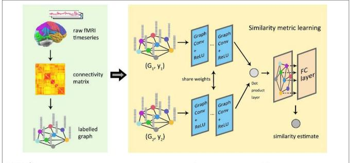
**FIGURE 9** Similarity measure learning of graph neural network in functional brain graphs. The information contained in the fMRI image was integrated into the graph through the graph partition and connection matrix. Two graphs were, respectively, used as the input of the two graph convolutional networks with sharing parameters, and the output of the network was combined by the inner product layer. Finally, a fully connected layer outputs the estimated similarity between the graphs.
