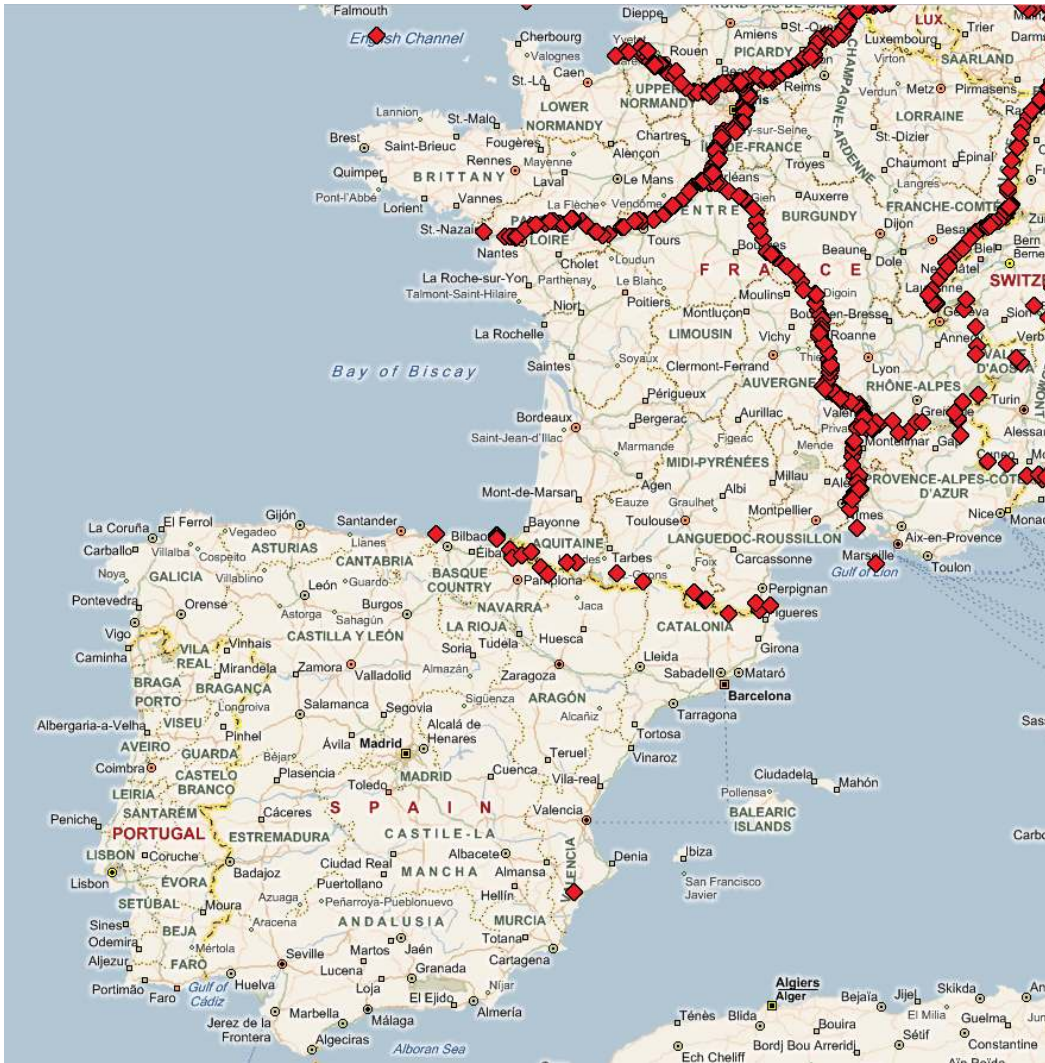
Figure 8: Partition generated by PUNCH. The input is the European road network, U is set to 1 000 000. PUNCH identifies the Pyrenees as natural cut.
