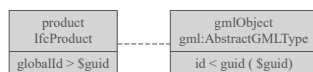
Figure 4. A rule converting a direct attribute to a direct attribute, here GlobalID in IFC to ID in CityGML.
