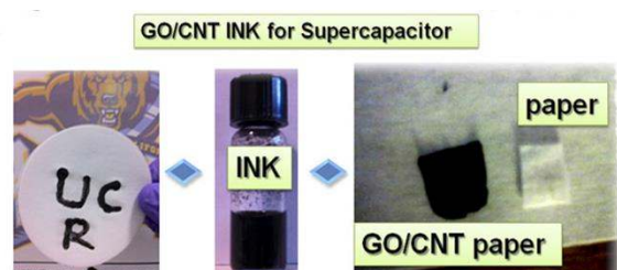
Fig.23. Preparation of supercapacitor electrodes using GO/SWCNT ink and paper. 112
