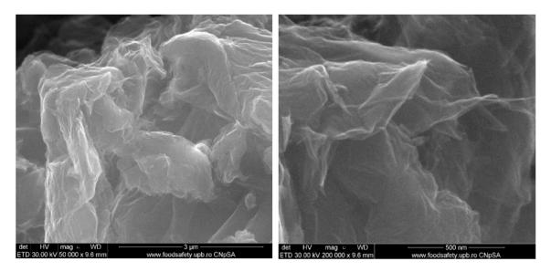
**Figure 2.** Microscopy analysis of a graphene oxide support morphology at 1000×, 10 kX. Reprinted from [116].
