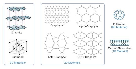
**Figure 1.** Chemical composition of graphene and processes in which it is involved. Graphene comprises a hexagonal carbon atom arrangement, which can form zero-, one-, and three-dimensional structures. Reprinted with permission from ref. [69]. Copyright 2012 American Physical Society.
