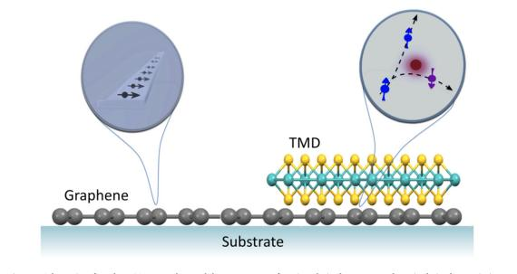
**Figure 6.** Schematics of graphene/TMD van der Waals heterostructures for spin polarized transport and manipulation by proximityinduced effects. The aim is to exploit the long spin coherence length of graphene and high spin–orbit coupling of TMDs/graphene interfaces in a single device.
