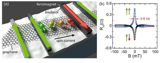
**Figure 1.** (a) Schematics of the typical four-terminal spin valve geometry for measuring spin lifetime in graphene samples. (b) Hanle experimental curve from which spin lifetimes are extracted using a semiclassical spin diffusion equation. Reprinted with permission from [14]. Copyright 2014 American Chemical Society.
