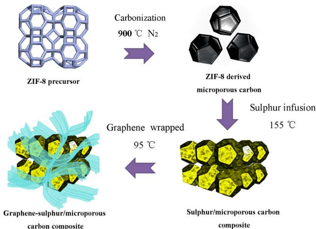
FIG. 1. Schematic illustration of the preparation of 3D hierarchically structured GS-S/C ZIF8-D composite.
