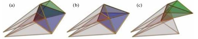
Figure 8: Elements that are adjacent to an element that has been split by a fracture plane must also be split to maintain mesh consistency. (a) Neighboring tetrahedra prior to split. (b) Face neighbor after split. (c) Edge neighbor after split.
