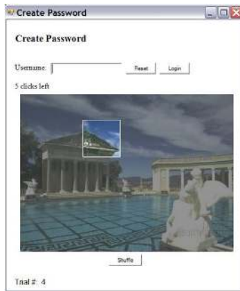
Figure 8: Persuasive Cued Click-Points. During password creation, users select a click-point from the highlighted viewport or press the shuffle button to relocate the viewport.
