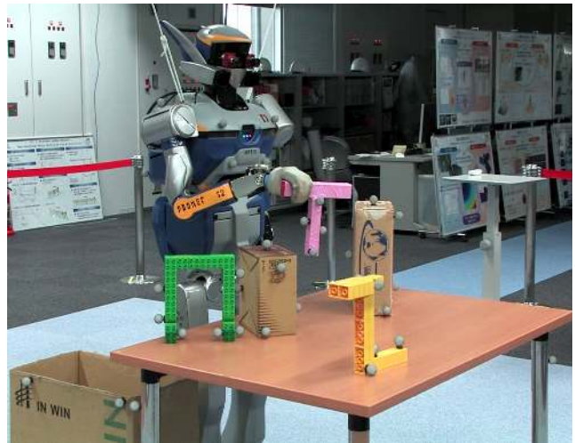
Fig. 1. The HRP2 lifting an object after executing one of the top-ranked grasps evaluated by the grasp-scoring function .
