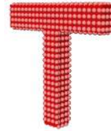
Fig. 4. An object (red) with sampled surface points (pink). Each surface point can be transformed to a set of grasps by using the point's position as \mathbf{P}_t and the surface normal at that point as \mathbf{P}_d .
