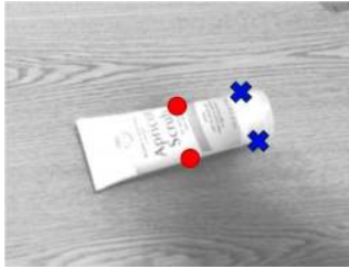
Fig. 2. Possible finger placements on an object. To be more robust to slippage, the "o's" are more desirable than the "x's".
