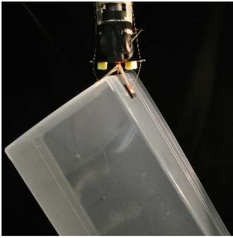
Fig. 5: When the gripper is used to grasp a flat-sided object, the film is straight. In this case there are no forces due to the curvature of the film, yet the gripper still holds the object.
