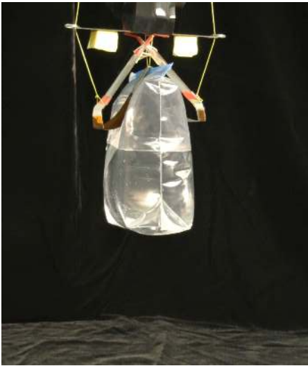
Fig. 19: Objects picked and placed by a robotic arm outfitted with the shear force gripper.
