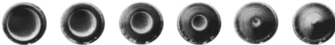
FIG. 12. Set of pictures taken from above each 2.7 ms ( R=20 mm, H=20 cm, and h=3 mm). These pictures correspond to the first points (before the arrow) in Fig. 11. It can be observed that a cavity forms and closes, producing a water jet (last picture).
