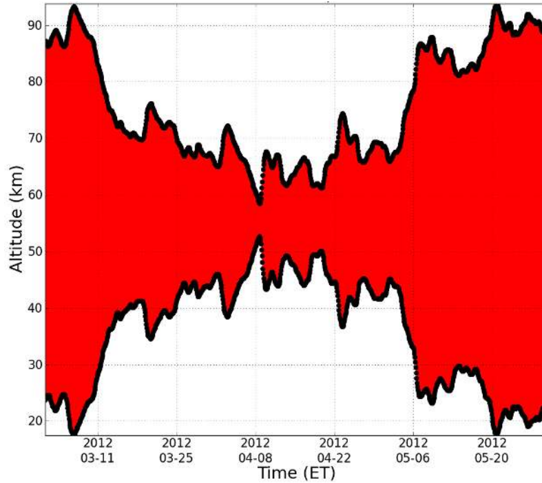
Figure S2. Orbital periapsis and apoapsis during GRAIL's PM. Altitudes are relative to the lunar mean radius of 1737.4 km (26) as measured by the Lunar Orbiter Laser Altimeter (47).
