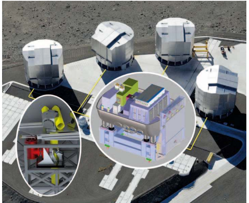
Figure 1. (Upper) GRAVITY at the VLTI Interferometer. GRAVITY combines the light from four UT or AT telescopes, measuring the interferograms for six base-lines simultaneously, with a maximum baseline of 200 metres. The insets depict the GRAVITY beam-combiner instrument (middle), which is located in the VLTI laboratory, and one of the four GRAVITY IR wavefront sensors (left) for each of the UTs.
