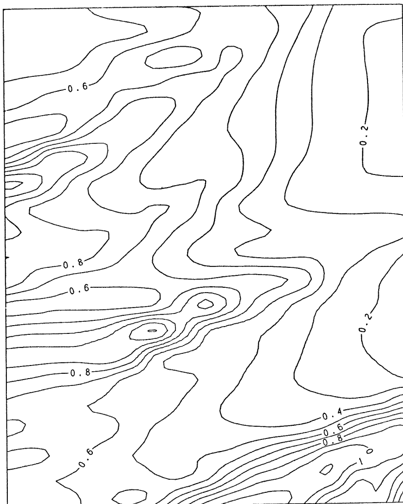
Figure 6.5. Amplitude contours, computed with complex phase function, in region R. No current influence.
