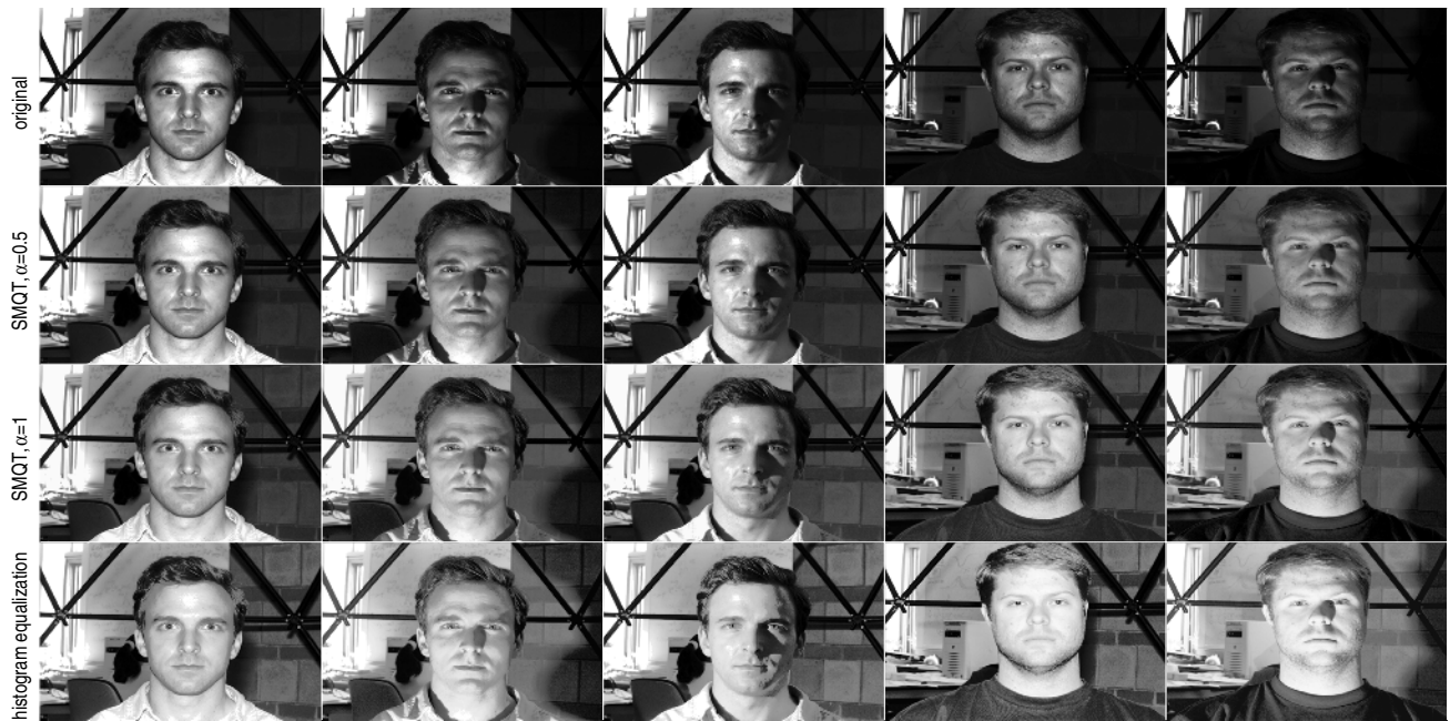
Fig. 5. Image enhancement results, part one. First row original image, second SMQT 8 of image blended with original image ( \alpha = 0.5 ), third SMQT 8 of image ( \alpha = 1 ) and fourth histogram equalization of image. Face images are from Yale Face Database B [8]. Zooming in the pdf images is recommended for detail studies. Note the differences of the forehead.
