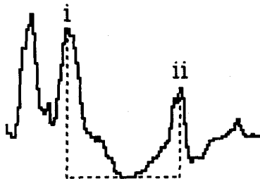
Figure 2. The amplitude of a peak is measured from the top of a peak to the lowest trough associated with that peak (e.g., the lowest trough for Peak i is to the right of that peak, whereas the lowest trough for Peak ii is to the left).
