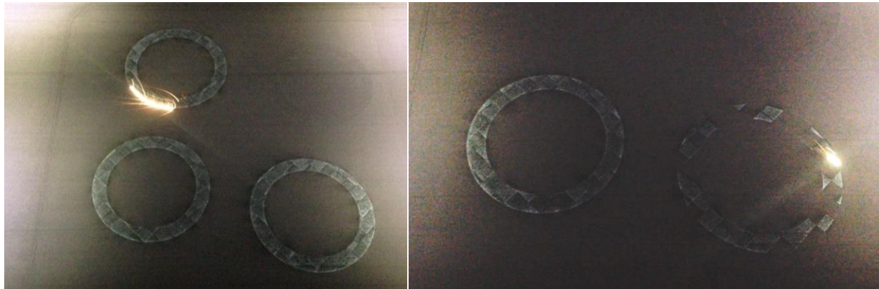
Figure 13. SLM Combustion Chamber Fabrication showing the Contouring (inside and outside edges) Pass (Left) and In-fill Pass (Right).
