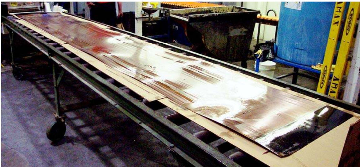
Figure 3.—GRCop-84 can be cold rolled with minimal difficulty. Large reductions without annealing are possible. GRCop-84 foil has been produced on an experimental scale.
