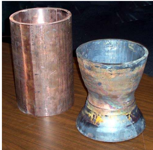
Figure 4.—GRCop-84 can be formed into shapes using conventional methods used for copper-based alloys. The cylinder shown on the left was bump formed from two pieces of a plate and friction stir welded together. Another cylinder was hot metal spun into the hourglass-shaped liner preform shown on the right.
