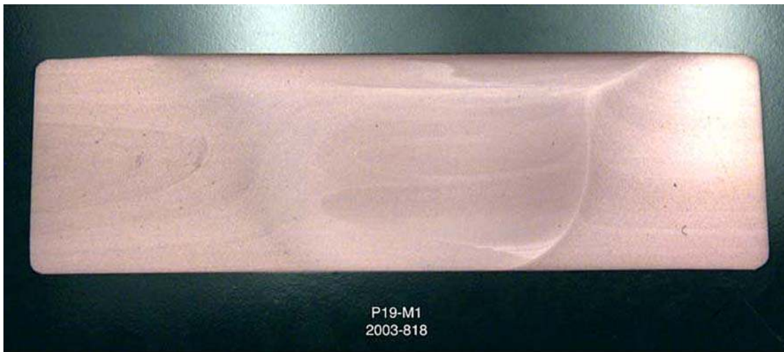
Figure 22.—Friction stir welding (FSW) of GRCo-84 has been developed at NASA Marshall Space Flight Center. GRCo-84 can be welded using a butt joint with ease by FSW. Unlike NARloy-Z, which did not exhibit a good weld, GRCo-84 shows full penetration and a void-free weld zone. GRCo-84 also has a wide processing window, which allows successful friction stir welding under a large variety of conditions. As shown in the tables below, the FSW welds retain almost all of the strength of the parent plate and can actually exceed the strength of the parent plate in some cases.
