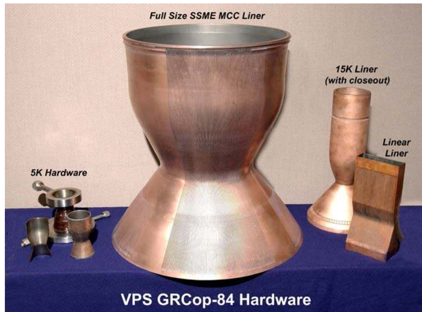
Figure 5.—In addition to extrusion and HIPing, GRCop-84 can be vacuum plasma sprayed (VPSed) into complex shapes. NASA Marshall Space Flight Center has successfully used VPS to produce many liner configurations including a full-scale space shuttle main engine (SSME) main combustion chamber (MCC) liner. A major advantage of VPS is the ability to introduce environmental and thermal barrier coatings on the hot wall as a functional gradient material (FGM).
