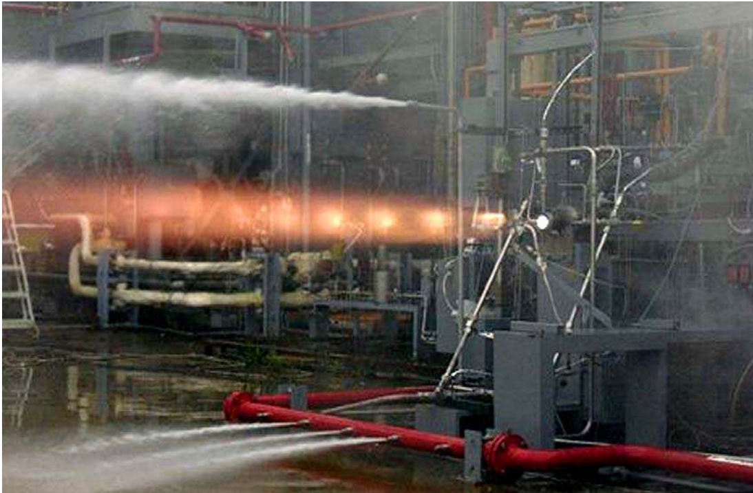
Figure 23.—NASA Marshall Space Flight Center produced and hot fire tested a GRCop-84 5000-lb thrust cell with a NiCrAlY functionally graded material on the hot wall. Despite two injector failures and 108 hot fire tests, the NiCrAlY coating remained intact and showed no visible wear or degradation. Hot wall cracks were produced in similar NARloy-Z liners tested in the 1970s. No such cracks were observed in the GRCop-84 liner even though it was tested at a higher hot wall temperature. The liner was also tested at a stoichiometric oxygen to hydrogen ratio, which would degrade an uncoated NARloy-Z liner in a few seconds due to blanching with no detectable damage. The GRCop-84 liner survived eight stoichiometric hot fire tests.
