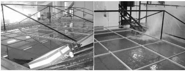
Fig. 2. Pictures from the three dimensional physical model. On the left, solid block landslide model and wave tank. On the right, impact of the landslide model with water.
