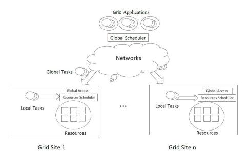
Figure 2. GFA IoT Grid Task Scheduling Architecture.
