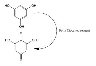
Figure 2. Redox reaction between polyphenols and Folin Ciocalteu reagent.
