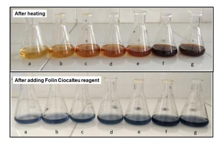
**Figure 1.** Tea extract after heating for 20 min and after the addition of Folin Ciocalteu reagent at: (a) 28; (b) 50; (c) 60; (d) 70; (e) 80; (f) 90; and (g) 98  $^{\circ}$ C.
