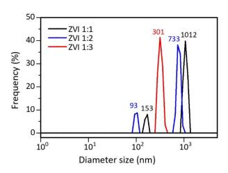
Figure 4. PSA results for ZVI particle size distribution.
