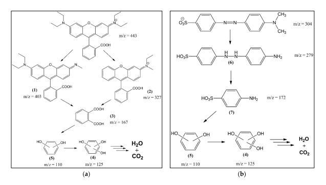
**Figure 11.** Schematic illustration of the proposed degradation pathway of: (**a**) rhodamine B; and (**b**) methyl orange.
