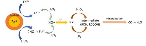
Figure 10. Mechanism of heterogeneous Fenton reactions with ZVI.
