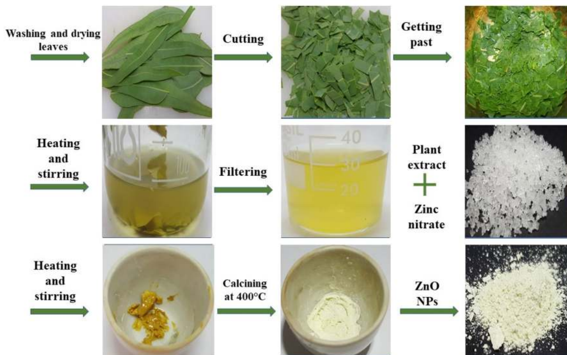
Fig. 4 Schematic representation of ZnO NPs synthesis using the leaf extract of Eucalyptus globulus Labill. and zinc nitrate hexahydrate
