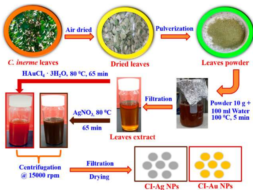
Figure 1. Schematic showing extract preparation and green synthesis of CI-Au and CI-Ag nanoparticles (NPs) using aqueous leaves extract of Clerodendrum inerme .
