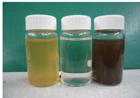
FIGURE 1: Apple extract, aqueous solution of 0.1 M AgNO 3 , and synthesized AgNPs (from left to right).
