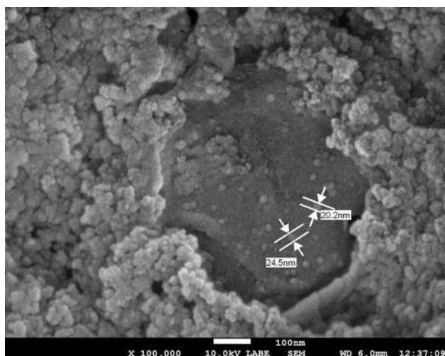
Fig. 6 SEM image displaying spherical shape of biosynthesized AgNPs
