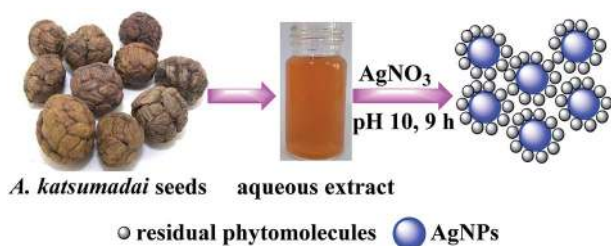
Scheme 1 Schematic of the green synthesis of AgNPs using Alpinia katsumadai seed extracts as the bioreductant.
