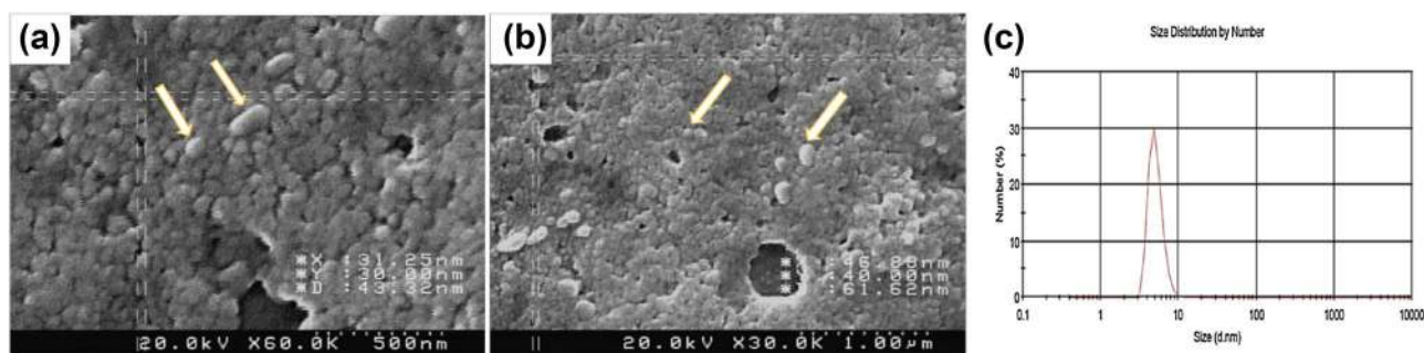
Fig. 4 a) FESEM images scale in a 500 nm and b 1 \mu\text{m} . Nanoparticles coated with organic materials of plant extract have been indicated with arrows in two pictures c particle diameter analysis from Ag NPs biosynthesized by S. spinosa extract
