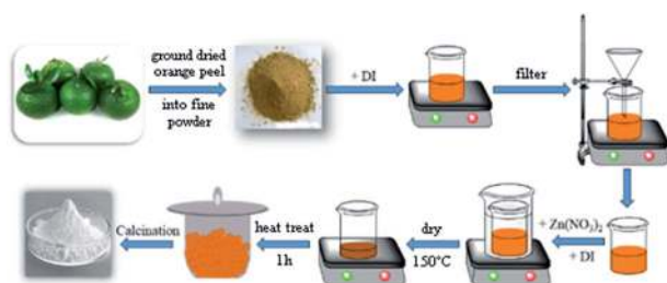
Fig. 1 Schematic diagram of the green synthesis of ZnO nanoparticles (ZnO NPs).
