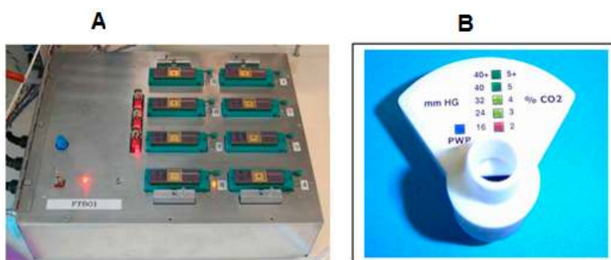
Figure 11. (A) Functional test board (FTB) loaded with eight packaged die containing functionalized NTFET devices. (B) Mockup capnography device. Reproduced with permission from reference [28].
