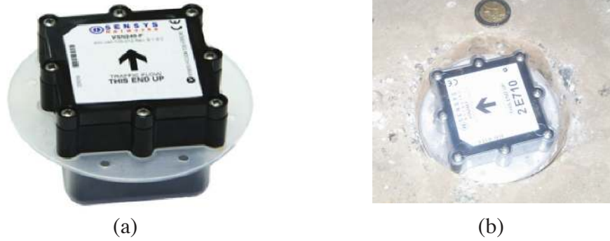
Figure 4. Magnetic sensors. (a) Sensys Networks VDS240 protected by a hardened plastic case (With permission of Sensys Networks, Inc.); (b) A magnetometer in its final location in the south ring, about 3 cm below the road surface, before being covered with fast-drying epoxy (the arrow points in the direction of traffic flow). A 2 Euro coin is shown near the sensor for comparison: the actual size is 7.4 cm × 7.4 cm × 4.9 cm and the weight is 300 grams.
